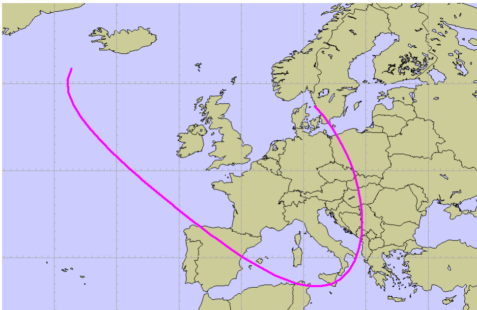
Figure 21 Geodetic arc centred on London; x-radius 1000km, y-radius 2000km, rotation 45°.
